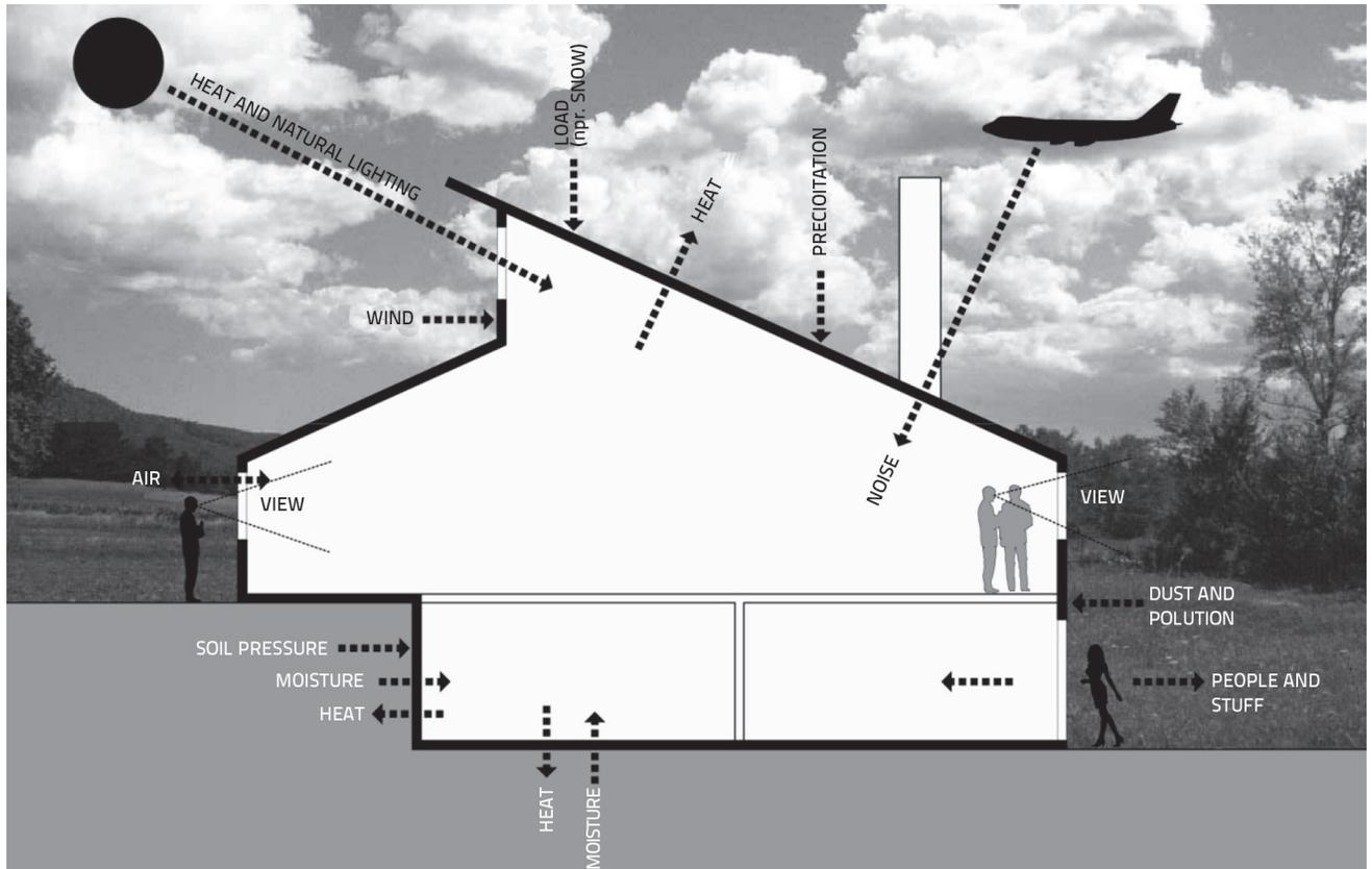
Figure 7. Impact of external environment on building envelope
