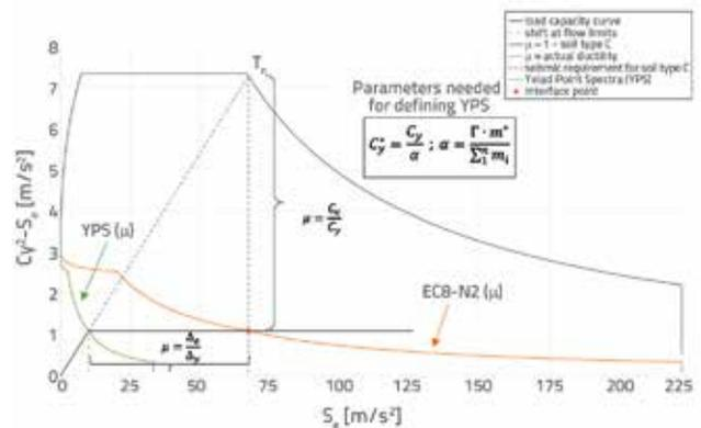
Figure 2. YPS and N2 response spectra for the city of Zagreb with ground accelerations of  $a_g = 2.55 \text{ m/s}^2$  and foundation soil type C in ADRS format for identical ductility factor
