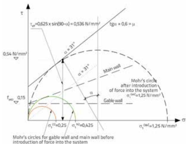
Figure 36. Stress at the joint of gable wall and load bearing wall before introduction of additional force into the system, represented by Mohr's circles, and stress after an increase in stress at the joint to approximately 50% of limit wall capacity = approximately 1.25
