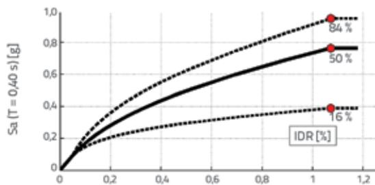
Figure 19. Fractile of IDA curves in the format of spectral acceleration as a function of period T = 0.4s and displacement at the top of the building in % as defined in Figure 18.
