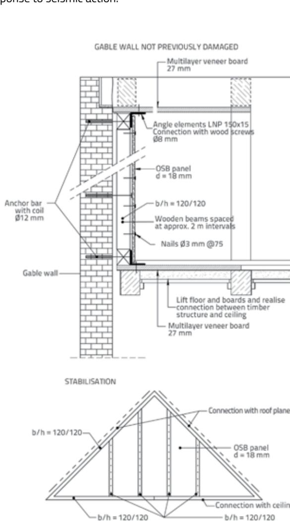
Figure 34. Proposal for stabilising gable wall that has not suffered damage in previous earthquakes, but reveals deficiencies with regard to connection with the floor structure and roof area
