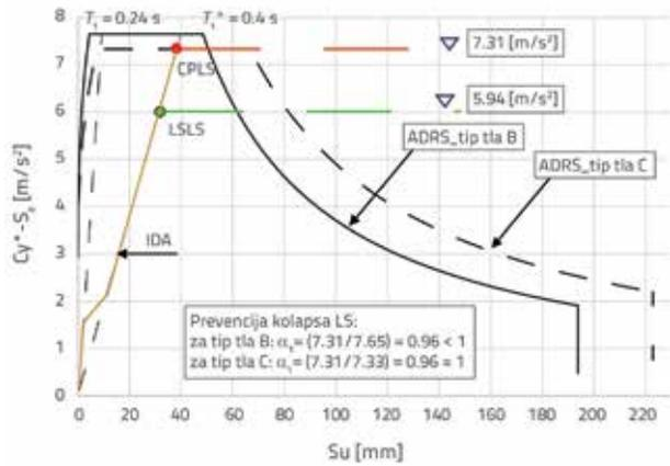
Figure 23. IDA curve with points of achievement of design limit states (LS and CP) and fulfilment factor obtained by IDA analysis for X-direction in ADRS format
