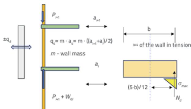
Figure 30. Wall model for determining critical horizontal acceleration, left, and distribution of stress along wall width, right
