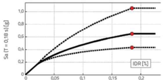
Figure 25. Fractile of IDA curves in the format of spectral acceleration as a function of period  $T = 0.18s$  and displacement at the top of the building in % as defined in Figure 24.
