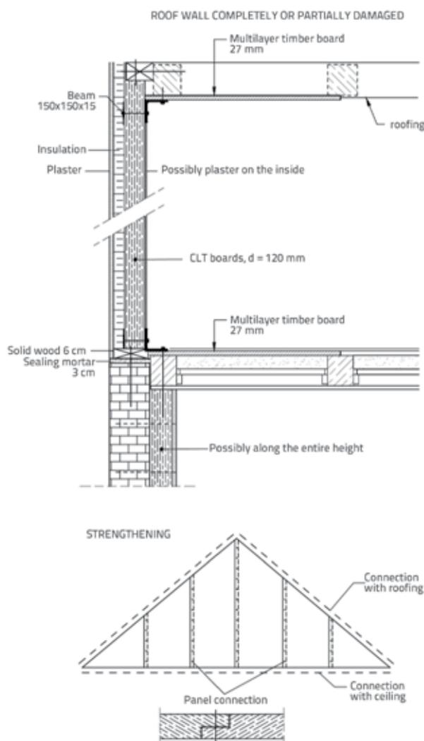
Figure 35. Proposal for improving gable wall with CLT-panels for walls that have been partly or fully damaged in previous earthquakes and must be removed
