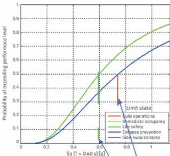
Figure 20. Fragility functions for two limit states. LS and CP
