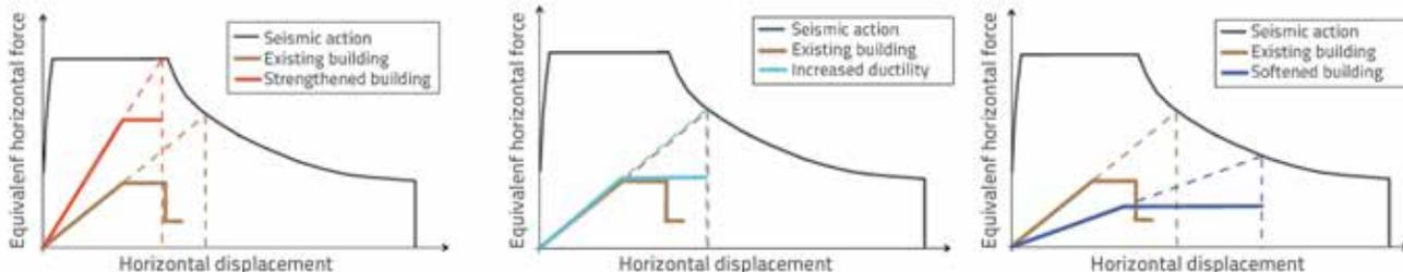
Figure 33. Three different strategies for improving structural response to seismic action: strengthening by increasing stiffness and bearing capacity (left), increase in ductility and deformation capacity (centre), and weakening (softening) of the structure e.g. by installing seismic isolators
