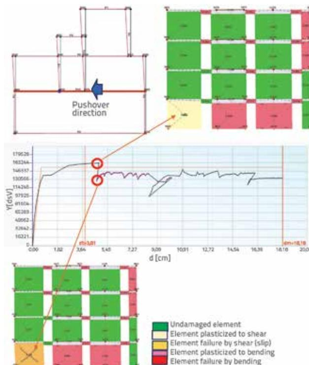
Figure 11. Failure mechanism of central wall in X-direction (analysis No. 3)
