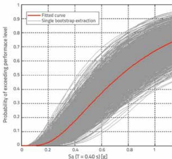
Figure 21. Visualisation of deviation of results for all seismic records as related to mean value
