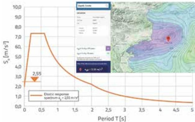
Figure 1. Elastic response spectrum for the city of Zagreb for ground acceleration of  $a_g = 2.55 \text{ m/s}^2$  and for the foundation soil type C in A-T (acceleration - period) format
