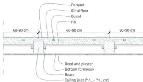
Figure 4. Floor structure of typical building
