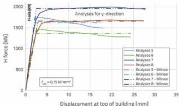
Figure 14. Pushover curve for Y-direction
