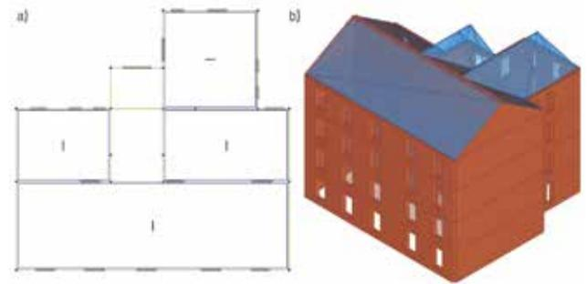
Figure 8. Plan view of replacement frames (left) and 3D model of the building (right)
