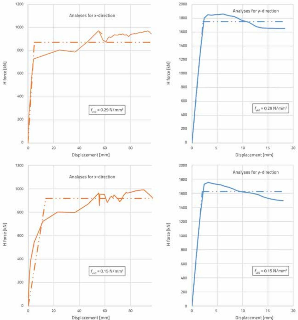
Figure 17. Curves obtained by pushover method for directions X and Y, and used as input for IDA analysis
