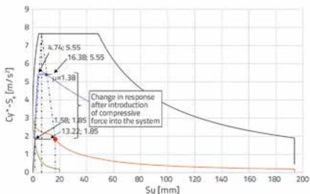
Figure 37. Example of change in response in case of design analysis No. 5 in Y-direction by introduction of prestressing force into the system
