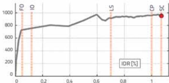
Figure 18. Definition of limit states on PO curve for X-direction
