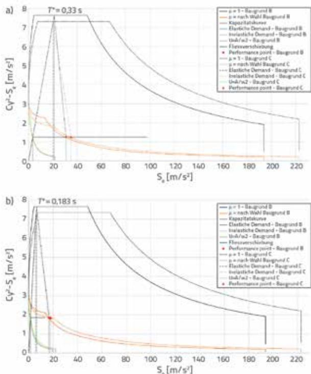
Figure 12. Results of the analysis No. 1 for X-direction (up) and analysis No. 5 for Y-direction (down) in ADRS format for the analysed building on soil type B and C, with wall mortar quality  $f_{vko} = 0.29 \text{ N/mm}^2$
