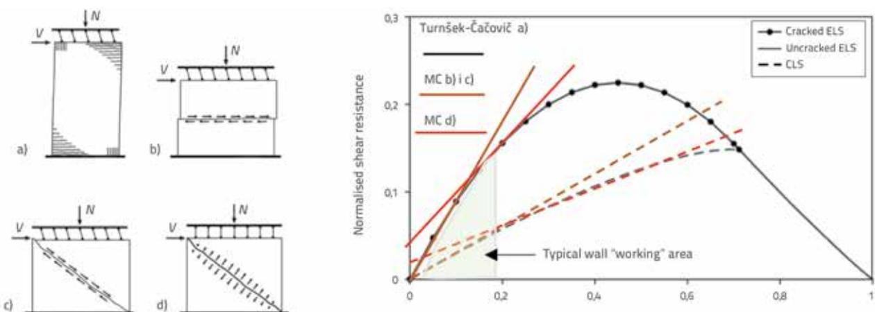
Figure 5. Constitutive models applied in program package 3muri: elastic limit of wall element (Turnšek-Čačovič a); Mohr-Coulomb failure condition b), c) and d). Solid line denotes ultimate limit state in the zone of elasticity, while dashed line denotes limit state of cracked wall element
