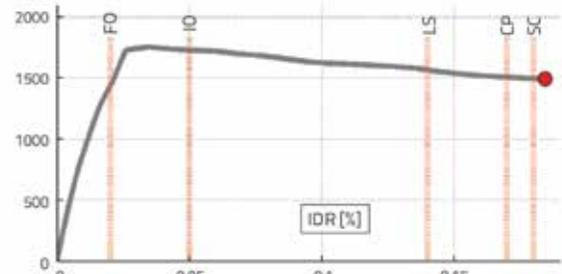
Figure 24. Definition of limit states on PO curve for Y-direction
