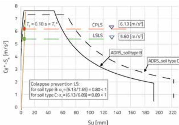
Figure 29. Fulfilment factor obtained by IDA analysis for Y-direction
