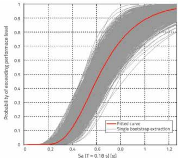
Figure 27. Visualisation of deviation of results for all seismic records as related to mean value
