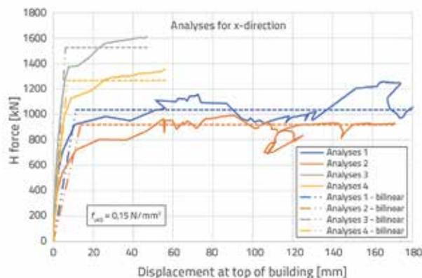
Figure 13. Pushover curves for X-direction
