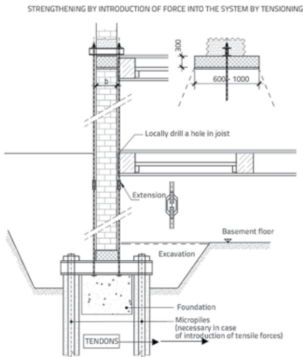
Figure 38. Example of introduction of force into the system by tendons and micropiles
