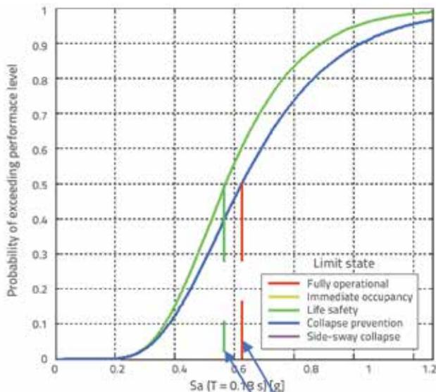
Figure 26. Fragility functions for two limit states, LS and CP
