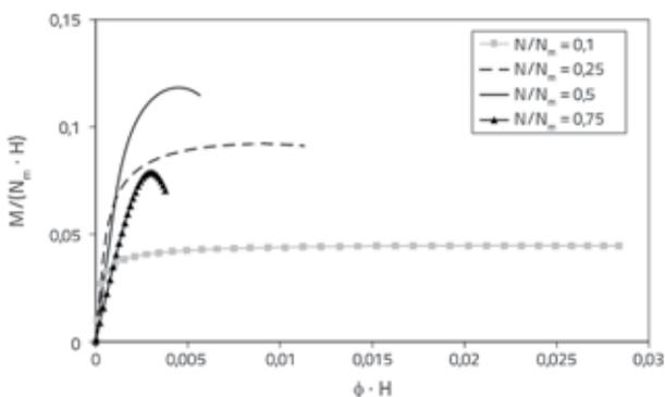
Figure 6. Dependence of bending moment (for Turnšek-Čačović constitutive model) on various levels of normal forces applied to masonry element, [9]
