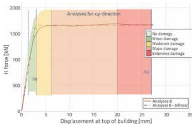
Figure 7. Qualitative presentation of damage due to displacement at the top of the building, according to [13]
