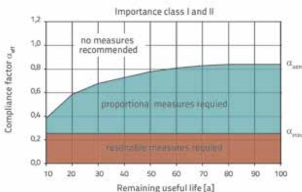
Figure 16. Recommended compliance factors as related to remaining useful life of buildings, according to SIA 269/8 [11]
