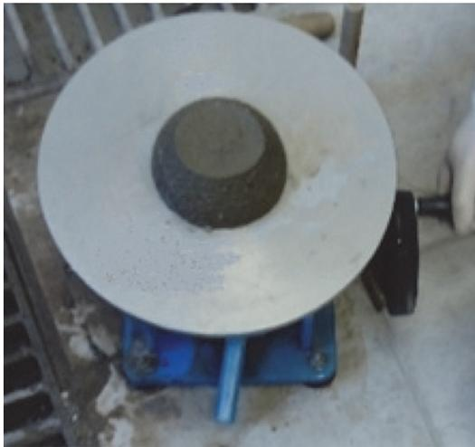
Figure 2. Flow table test
