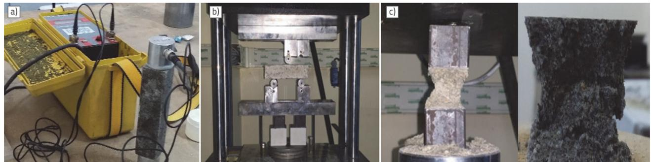
Figure 3. Experimental tests: a) UPV; b)  $f_f$ ; c)  $f_c$
